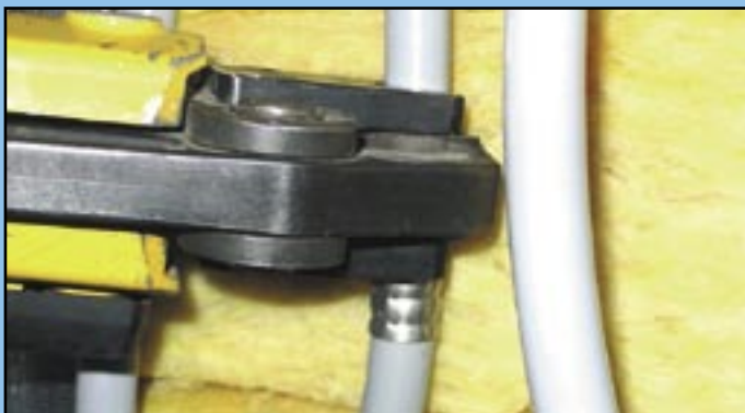
SLIDING SLEEVES AND PRESS FITTING SYSTEMS. Safer, faster as well as an undetachable connection / Manufacturer-independent - according to EN certifications - homologations
